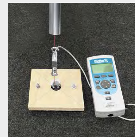
Testing of fixing element strength
